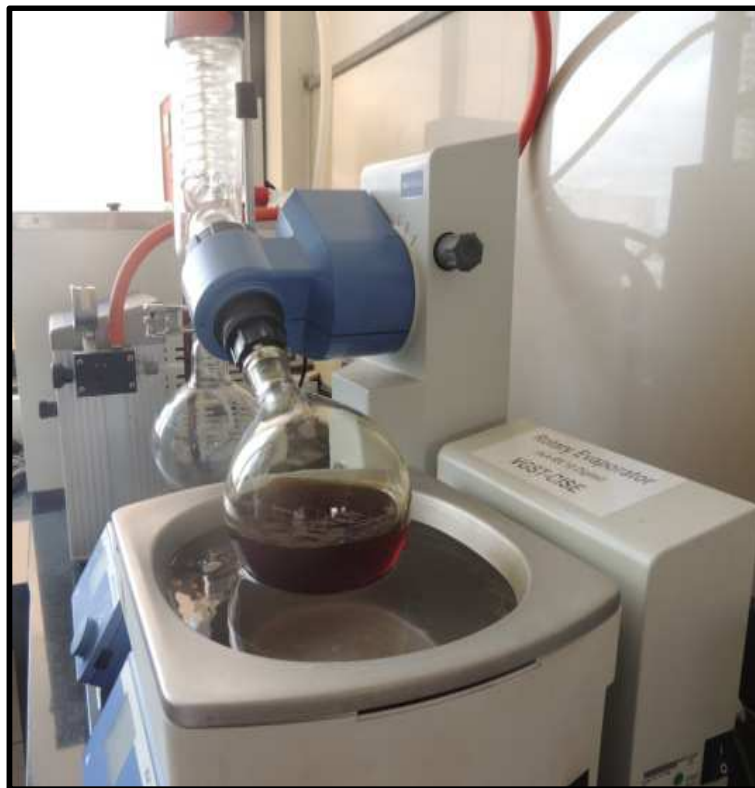
Photograph no 6: IKA Rotary evaporator to extract ethanol from crude extract
