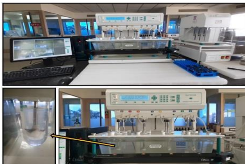
Figure 7: Dissolution testing apparatus (Electrolab, EDT-08LX) equipped with low volume conversion kit (EDT-08L/08L x 150 ml)
