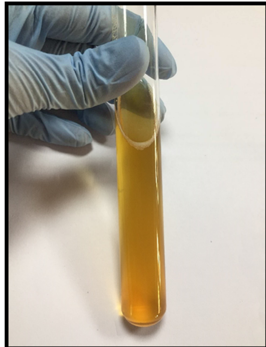
Figure 20: Ferric chloride test- Appearance of yellow color +ve for Coumarin glycoside
