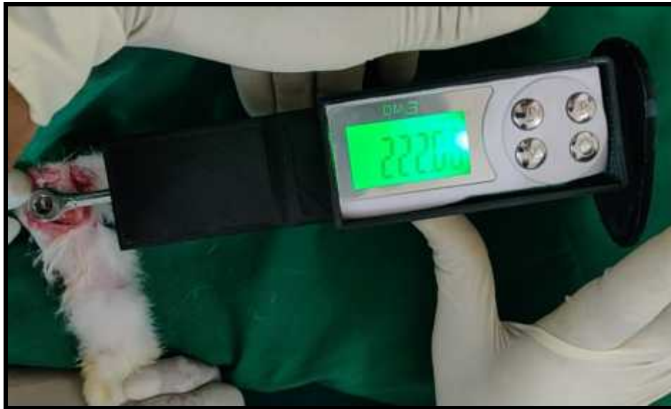
FIGURE 28: MEASUREMENT OF REMOVAL TORQUE QUOTIENT USING A CUSTOMIZED CALIBRATED, ELECTRONIC REMOVAL TORQUE WRENCH.
