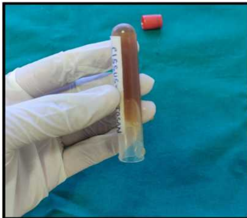
FIGURE 4: EVALUATION OF THIXOTROPIC BEHAVIOUR OF THE PREPARED HYDROGEL BY VIAL INVERSION METHOD.
