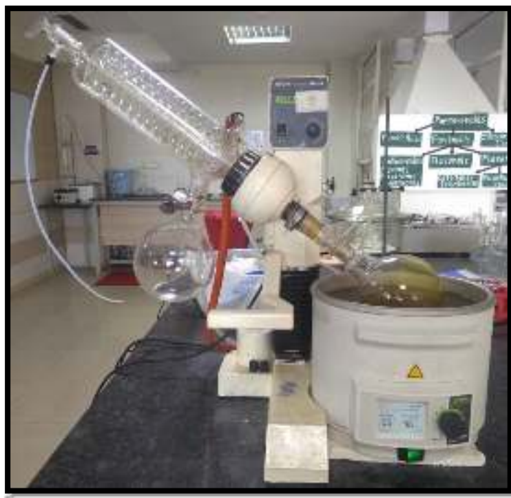
Fig 4: Evaporation of crude extract using rotary evaporater
