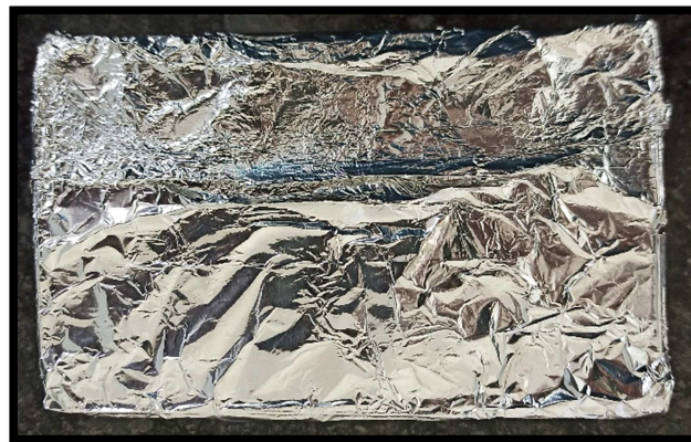
Culture plate covered with aluminium foil as MTT reagent is photosensitive
