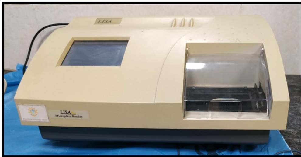
Fig 11: Microplate spectrophotometer (LISA Plus; 630nm)
