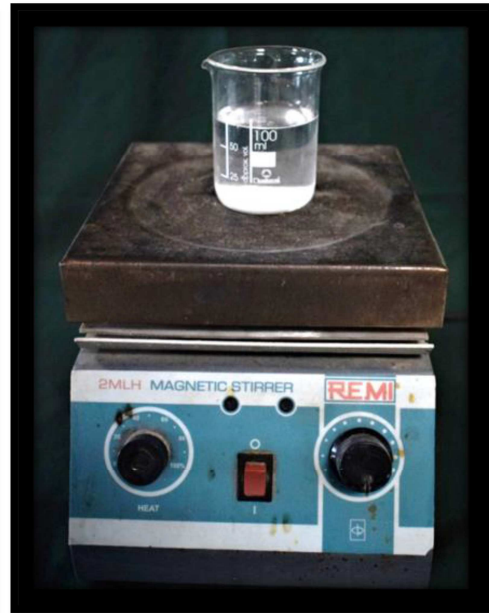
Fig 11: Magnetic Stirrer used to get a 0.2% Chitosan solution.
