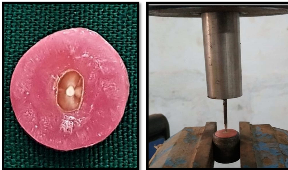
Fig 16: Pushout bond strength testing using a Universal testing machine at a cross head speed of 1mm/min
