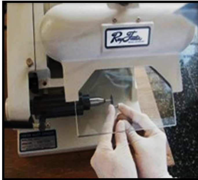
Fig 5: Samples decoronated at the level of CEJ using Diamond disc
