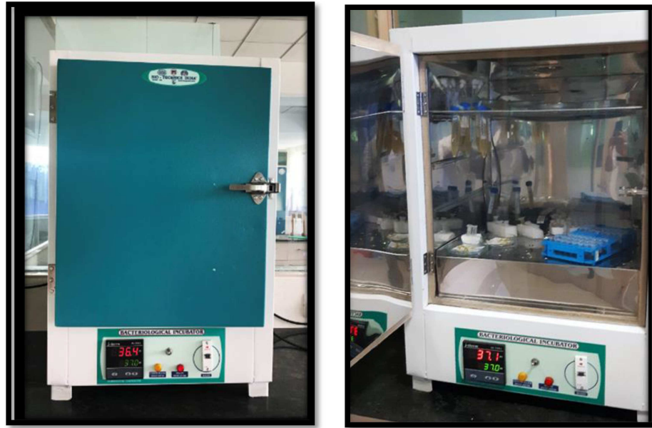
Fig 15: Storage of dentin discs in incubator at 100% humidity and 37 0 C.
