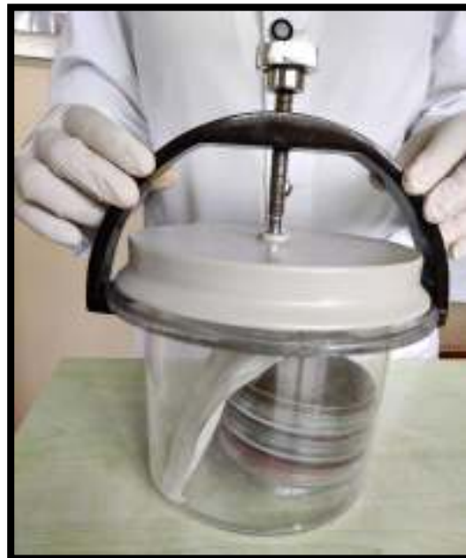
Photograph.8: Anaerobic Gas-Pak jar system was used to create an oxygen-free environment for the growth of anaerobic microorganisms.
