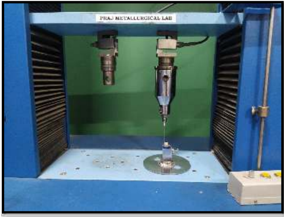
FIGURE 10 : Sample subjected to load for measuring the shear bond strength
