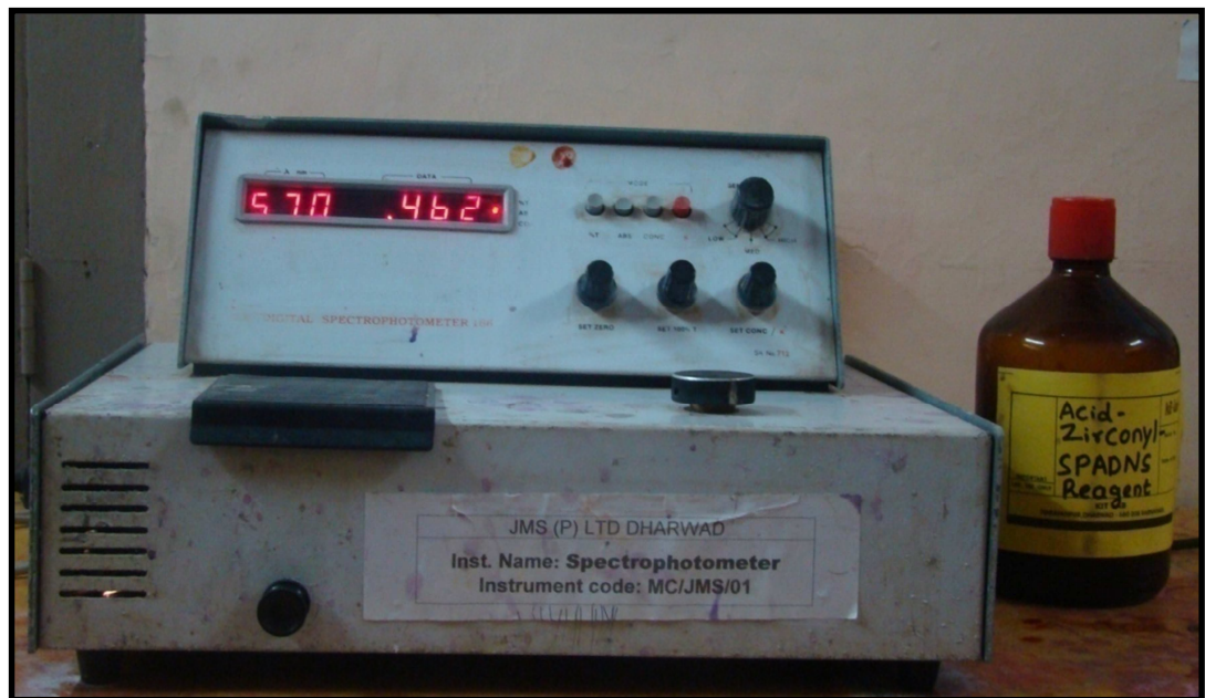
Photograph 2: Spectrophotometer and Acid Zirconyl - SPANDS reagent
