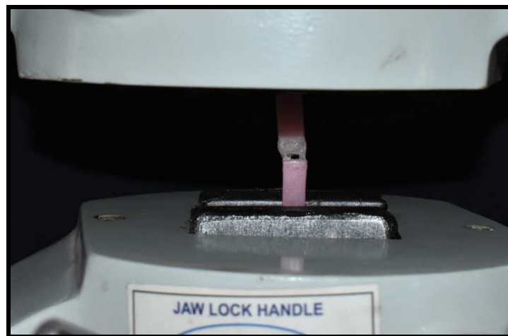
Figure 20: A rectangular Test Specimen of Size 40 mm x10 mm x7 mm.
