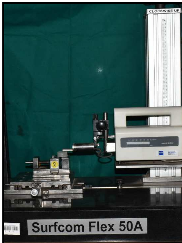
Figure 16: Profilometer Used To Check Surface Roughness
