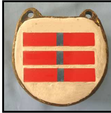
Figure 19: A rectangular Test Specimen of Size 40 mm x10 mm x7 mm with a brass spacer of dimensions 10 mm x 7 mm x 3 mm in between the wax blocks fabrication.
