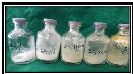
Figure 5: Various Concentration (1%,3%,5% and 7%) of Lawsonia inermis integrated with soft liner polymer.
