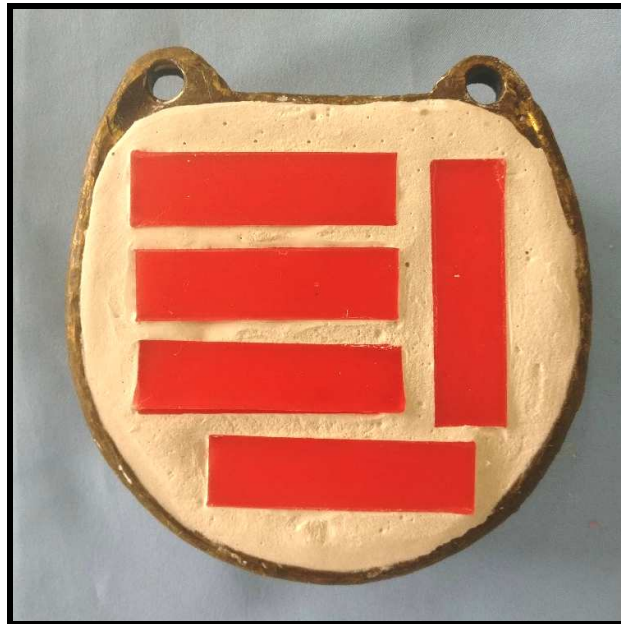
Fig. 4 Investment of wax blocks to obtain acrylic blocks
