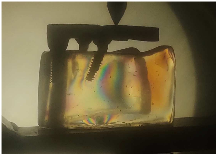
Fig 27. 3 rd order fringe at application of 180 N load on 5 mm cantilever length.
