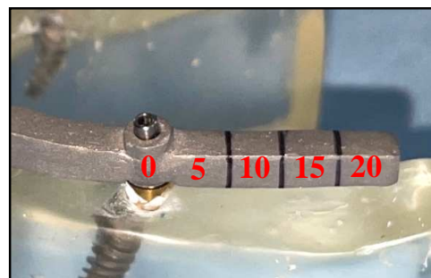
Fig 15. Markings at cantilever length of 5mm, 10mm, 15mm in the Co-Cr framework
