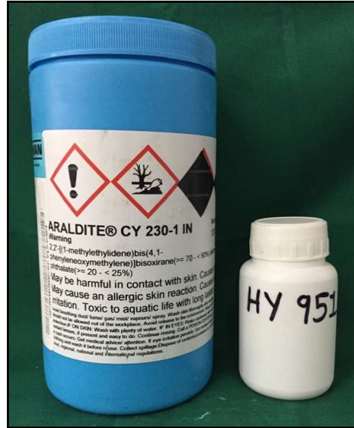
Fig 2. Adhesive CY 230 and Hardener HY 951 (Araldite casting system)
