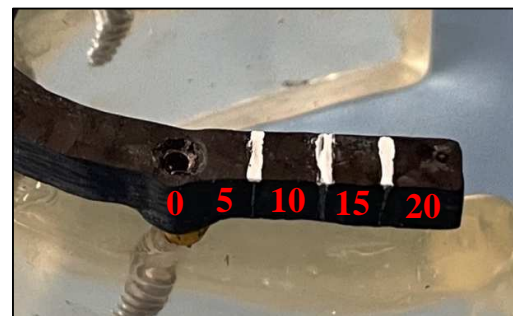
Fig 18. Markings at cantilever length of 5mm, 10mm, 15mm in the CFRC framework
