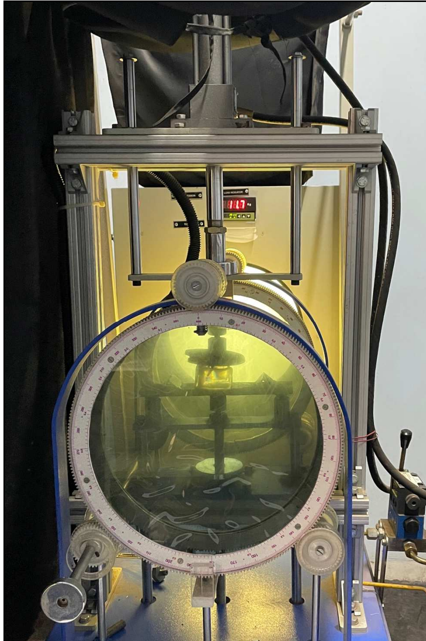
Fig 4. Model placed in the Circular polariscope (Model No. HP 12-02)
