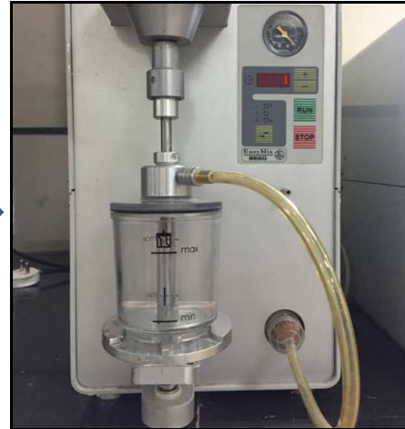
Fig 11. Vacuum mixing of the epoxy resin material CY230 and HY 951
