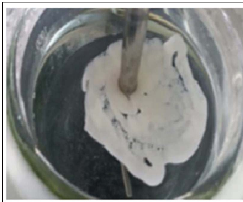
Figure 30: Gelation and floating property of the GRFS at 4 hours in 0.1 N HCl
