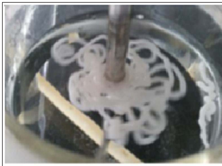
Figure 28: Gelation and floating property of the GRFS at 0 hour in 0.1 N HCl
