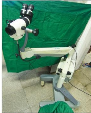
Figure 21. Colposcopy: A colposcope is a low-power, binocular field, stereoscopic microscope having a powerful light source that is used for magnified visual examination of the uterine cervix to diagnose cervical neoplasia. (133)
