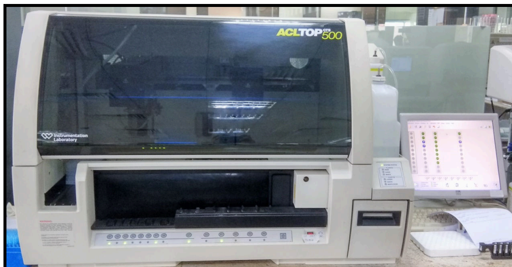
Photograph 5: Instrumentation Laboratory's ACL Top 300/500 used for estimation of PT, aPTT, D-dimer, fibrinogen levels
