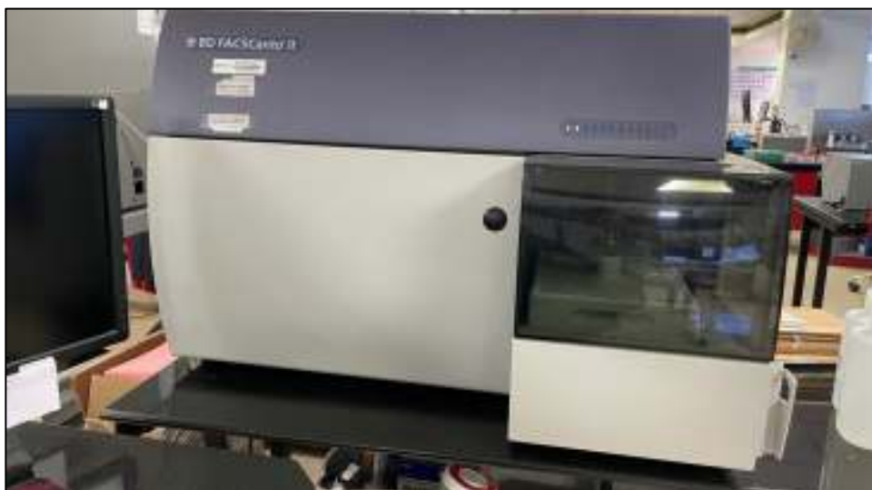
Figure 4. Becton Dickinson Facs Canto II Flow Cytometer
