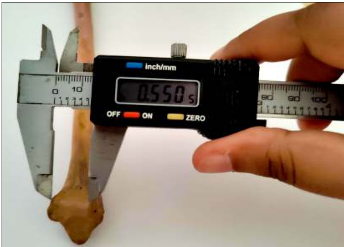
Photograph No. 10 : Measurement of the width of ulnar-notch of radius bone using digital vernier caliper .
