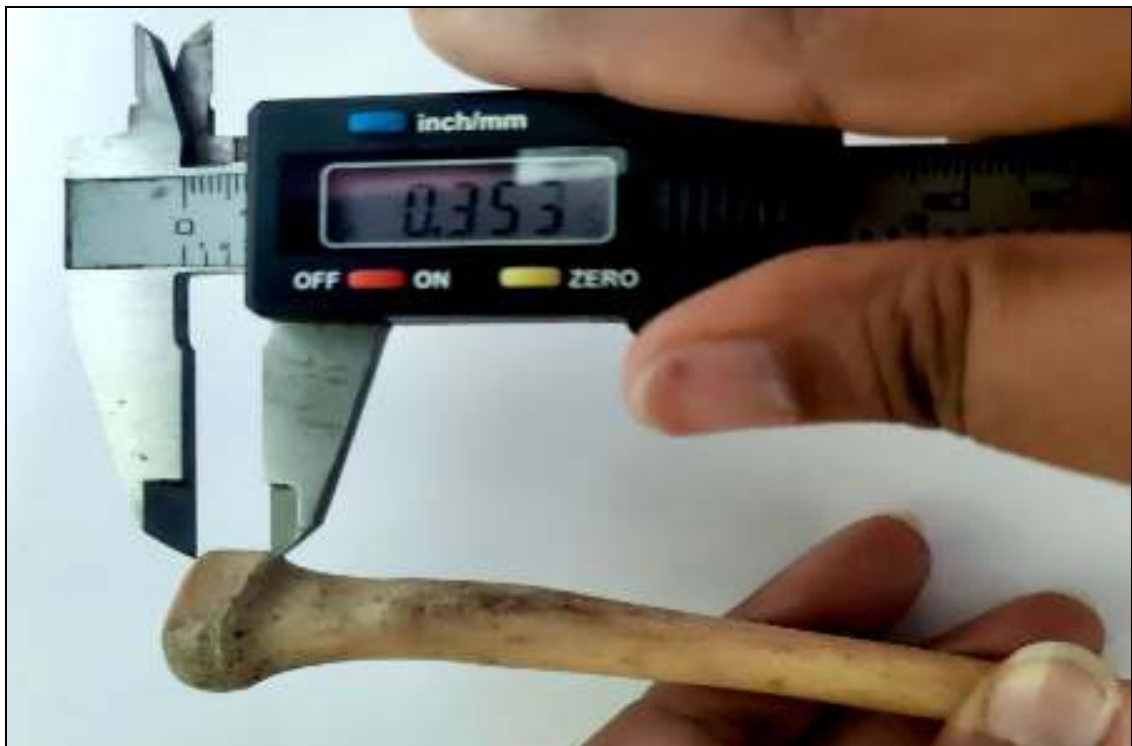
Photograph No. 4 : Measurement of the length of head of the radius bone using digital vernier caliper (R2).
