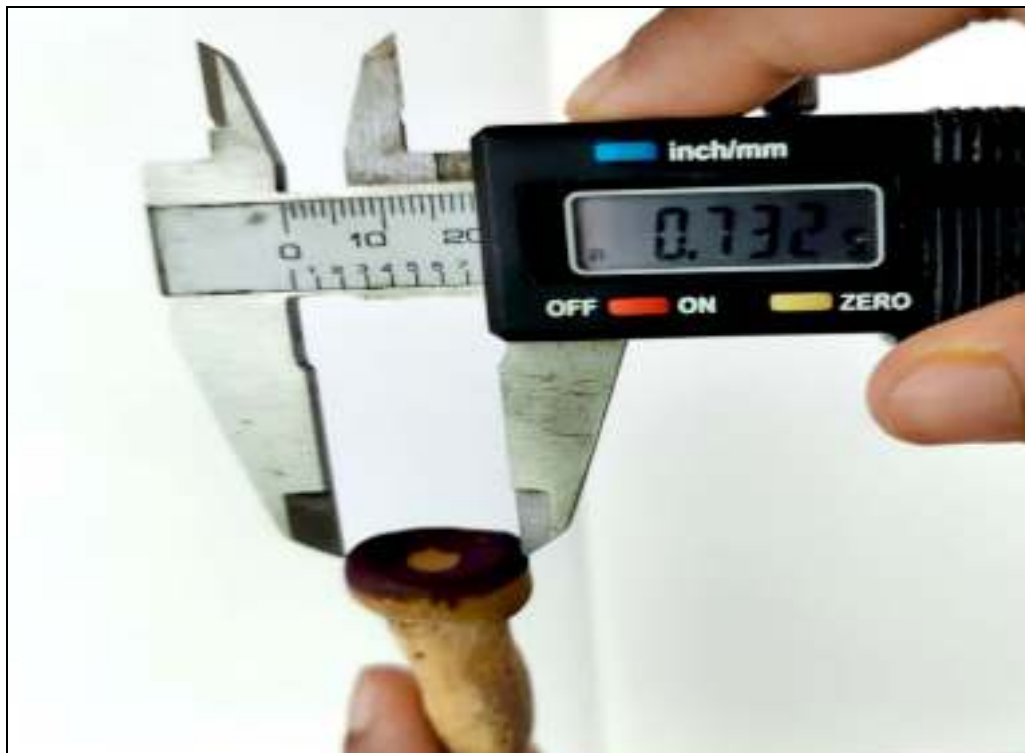
Photograph No. 5 : Measurement of the diameter of the head of the radius bone using digital vernier caliper.
