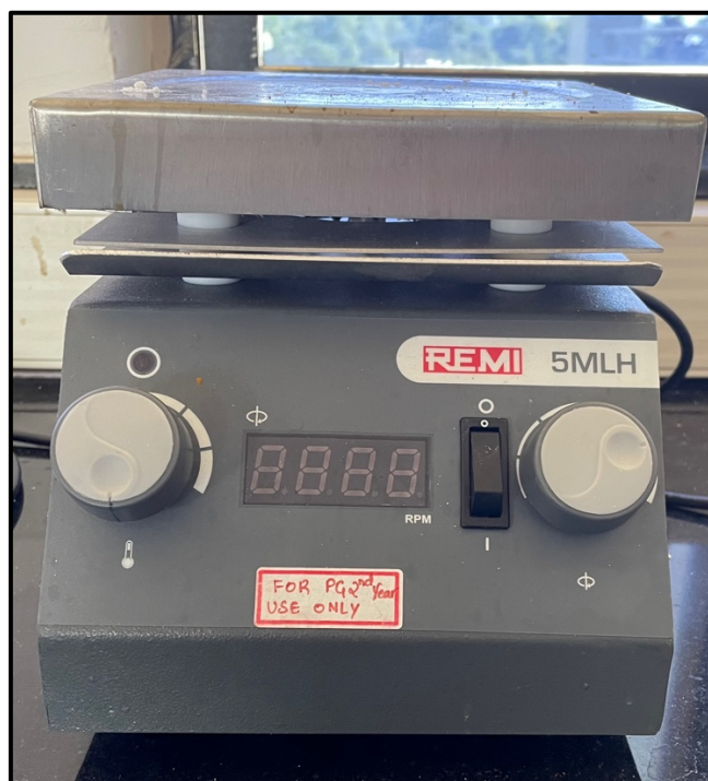
Figure No. 14: Photograph showing magnetic stirrer used for Herbal Dental gel preparation in the study.
