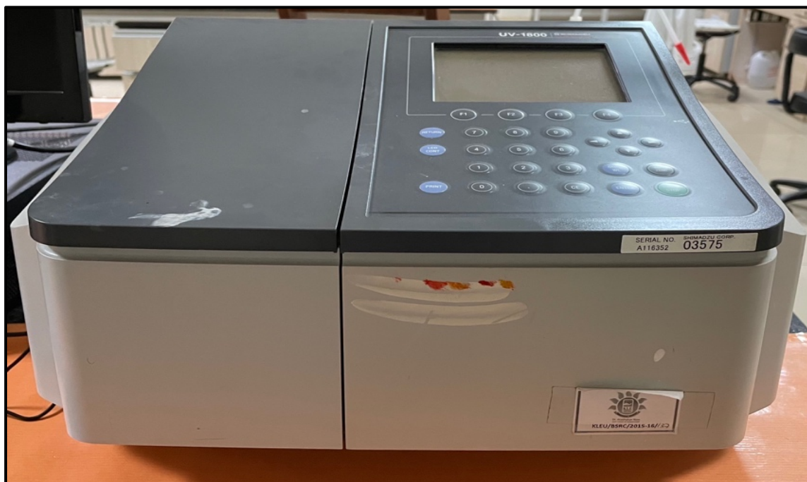
Figure No. 19: Photograph showing absorbance reader used for Time Kill Assay in the study.
