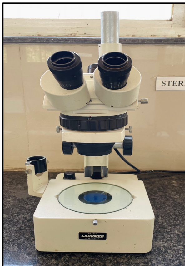
Figure No. 21: Photograph showing stereomicroscope used for evaluation of remineralization in the study.
