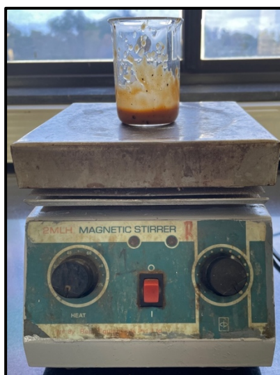
Figure No. 42: Photograph showing mixing of Carbopol gel solution with the mixture of the extracts on a magnetic stirrer.
