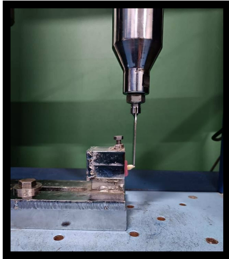
FIG 13. UNIVERSAL TESTING MACHINE WITH SPECIMEN UNDER SHEARING LOAD
