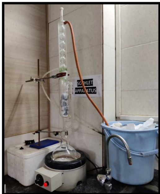
Soxhlet Apparatus for preparation of Ocimum basilicum crude extract
