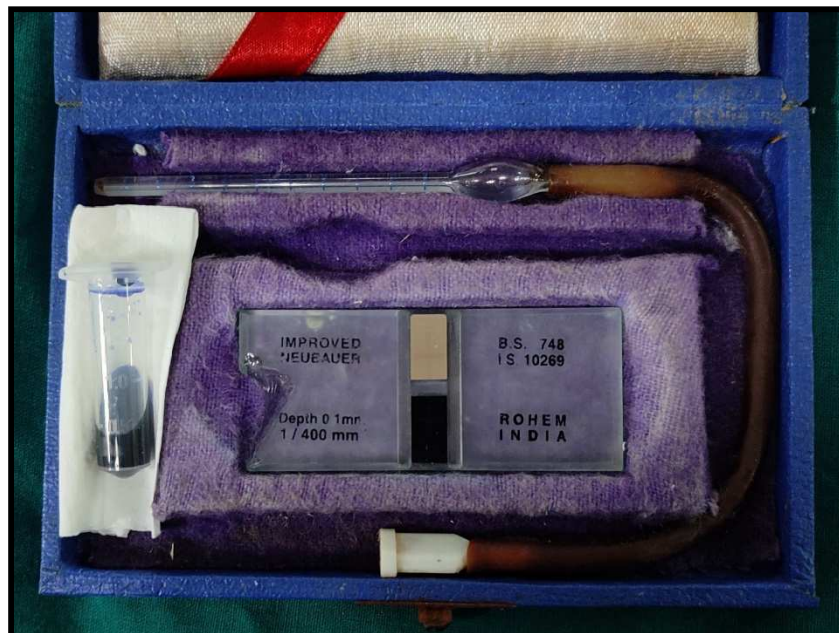
Fig 19: Haemocytometer with Trypan blue dye for cell attachment by Trypan blue assay
