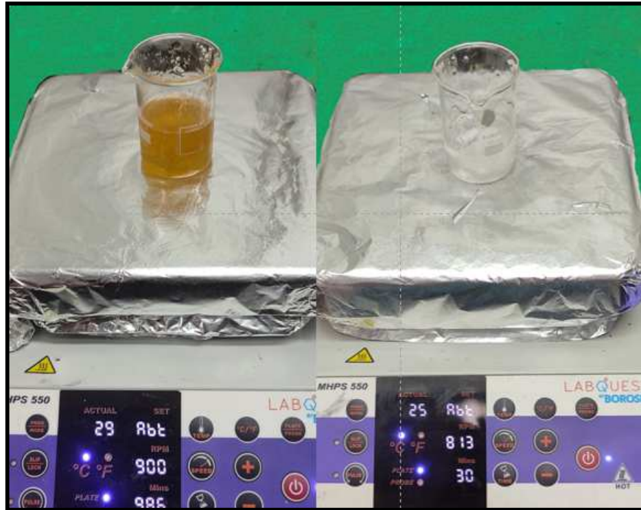
Fig 3: Chitosan and PEO solutions in 50 wt% aqueous acetic acid
