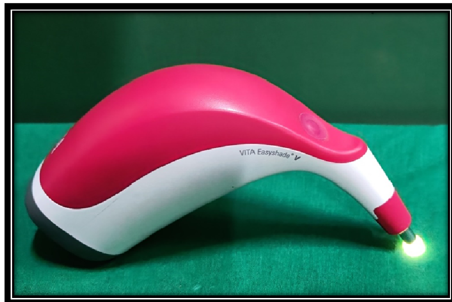
Figure 17: Spectrophotometer used for the determination of color stability of testing samples
