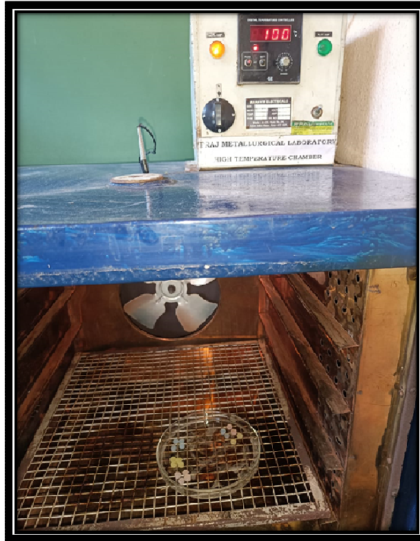
Figure 19: High temperature chamber used for accelerated aging showing specimens being subjected to 100 degree celsius
