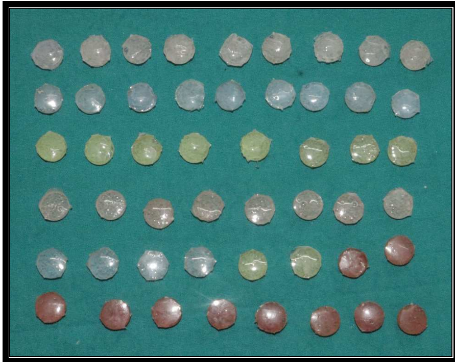
Figure 16: Coloured specimens of maxillofacial silicone to be used for the determination of color stability
