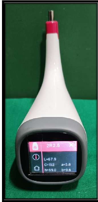
Figure 18: Spectrophotometer showing L*a*b* values
