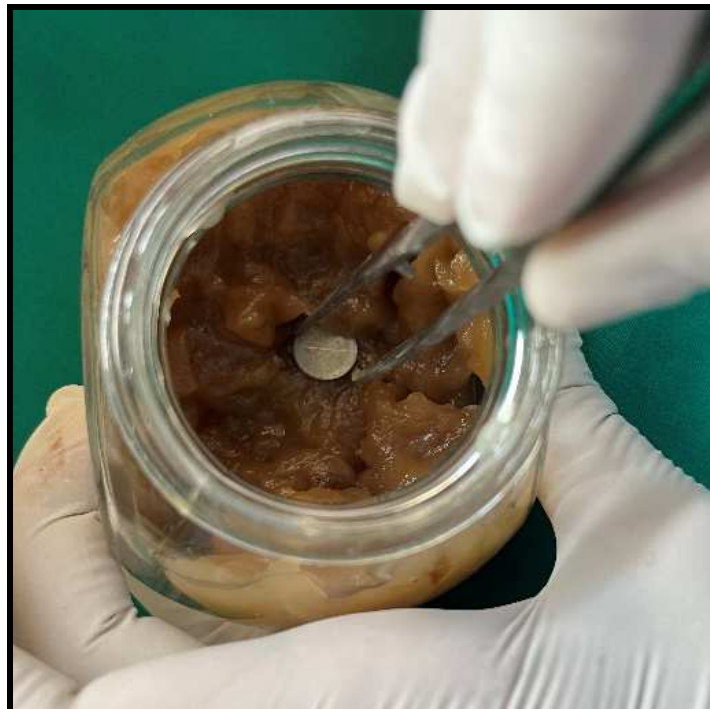
FIGURE NO 8: COATING OF TITANIUM DISC WITH HYDROGEL BY DIPPING METHOD
