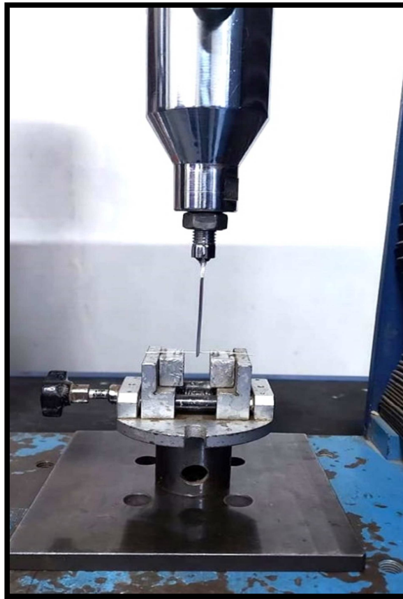
Fig.4.- Mounted wire on the lower jaw of the jig
