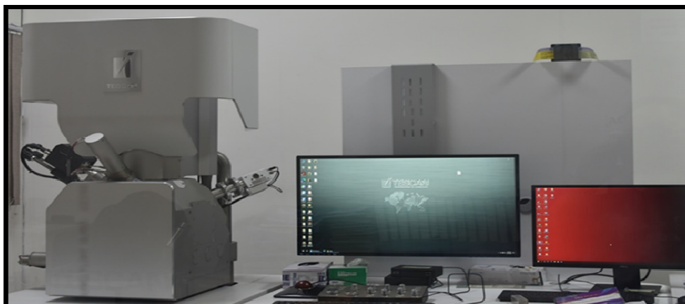
FIGURE-10 SCANNING ELECTRON MICROSCOPE- FESEM Zeiss EVO MA 10, Oxford INCA 250.
