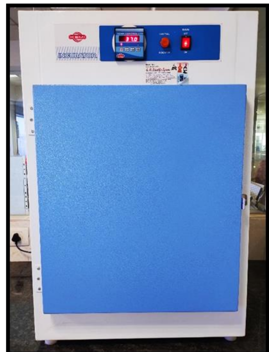
Photograph no. 4 – Microbiological Incubator, used for incubation of microorganisms.
