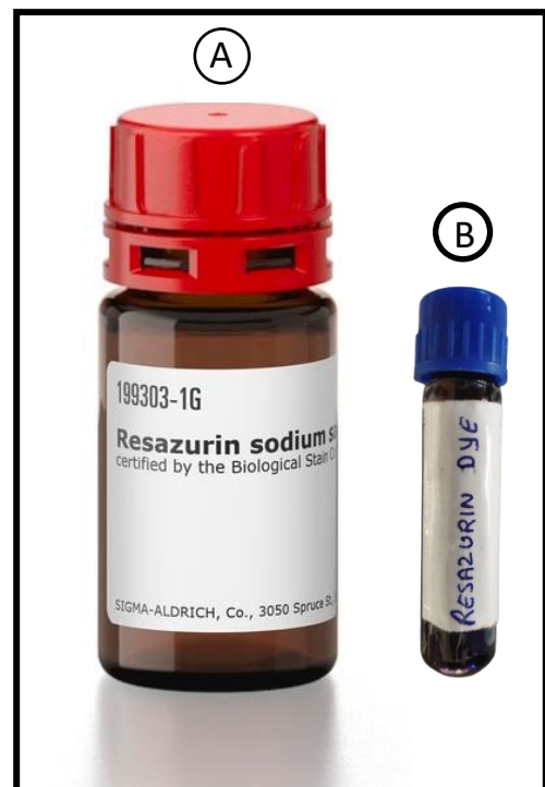
Photograph no. 8 - (A) Resazurin Dye Powder (B) – 0.015% of Resazurin dye prepared and used as indicator for Determination of MIC
