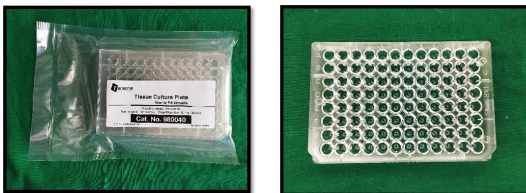
Photograph no. 12 – Sterile 96-well microtitre tissue culture plate, used for Broth Dilution Method to determine the MIC.
