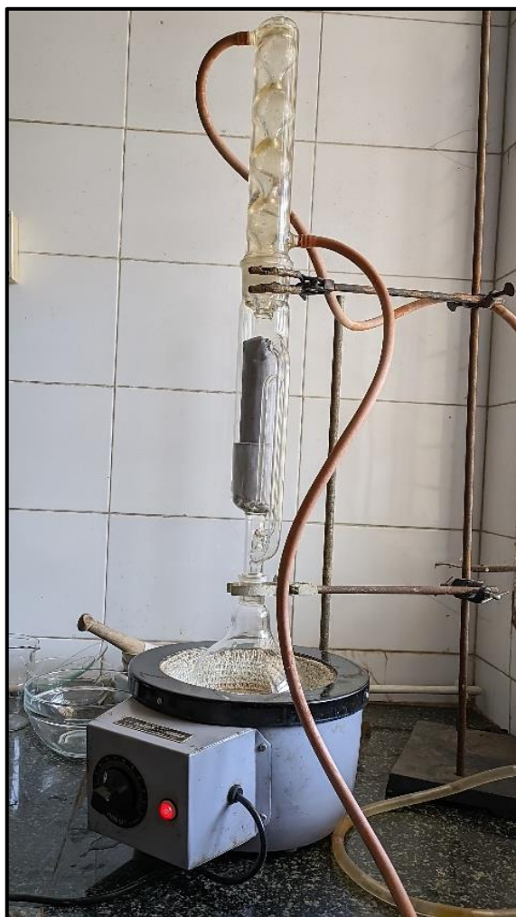
Photograph 4. Soxhlet Apparatus for preparation of Achyranthes aspera and Trachyspermum ammi crude extracts
