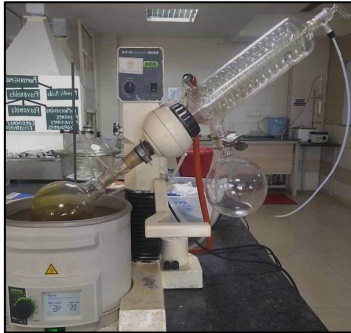
Photograph 5. IKA Rotary evaporator to extract solvent from crude extracts
