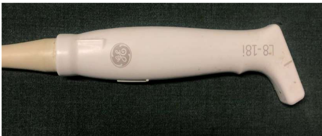
5-9 MHz L8-18i-D Linear array hockey stick ultrasound probe transducer
