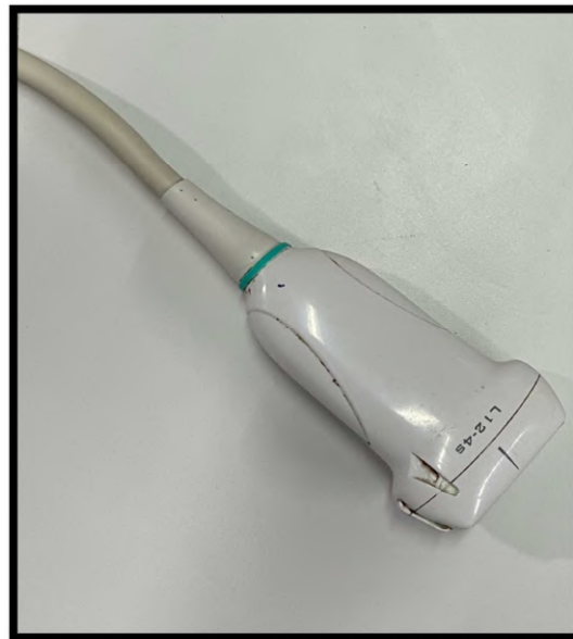
Fig 16: High frequency linear array transducer used for the study
