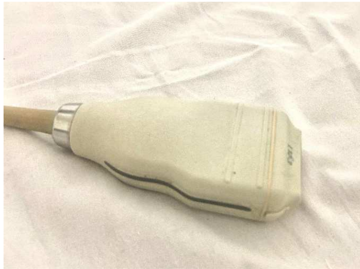
Fig 14: High frequency linear arrays transducers used for the study.
