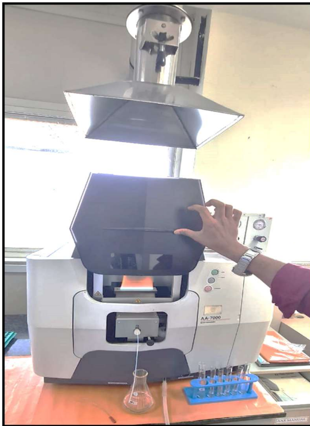
Photograph 4: THE DILUTED AND PREPARED SAMPLES BEING TESTED BY FLAME ATOMIC ABSORPTION SPECTROMETRY
