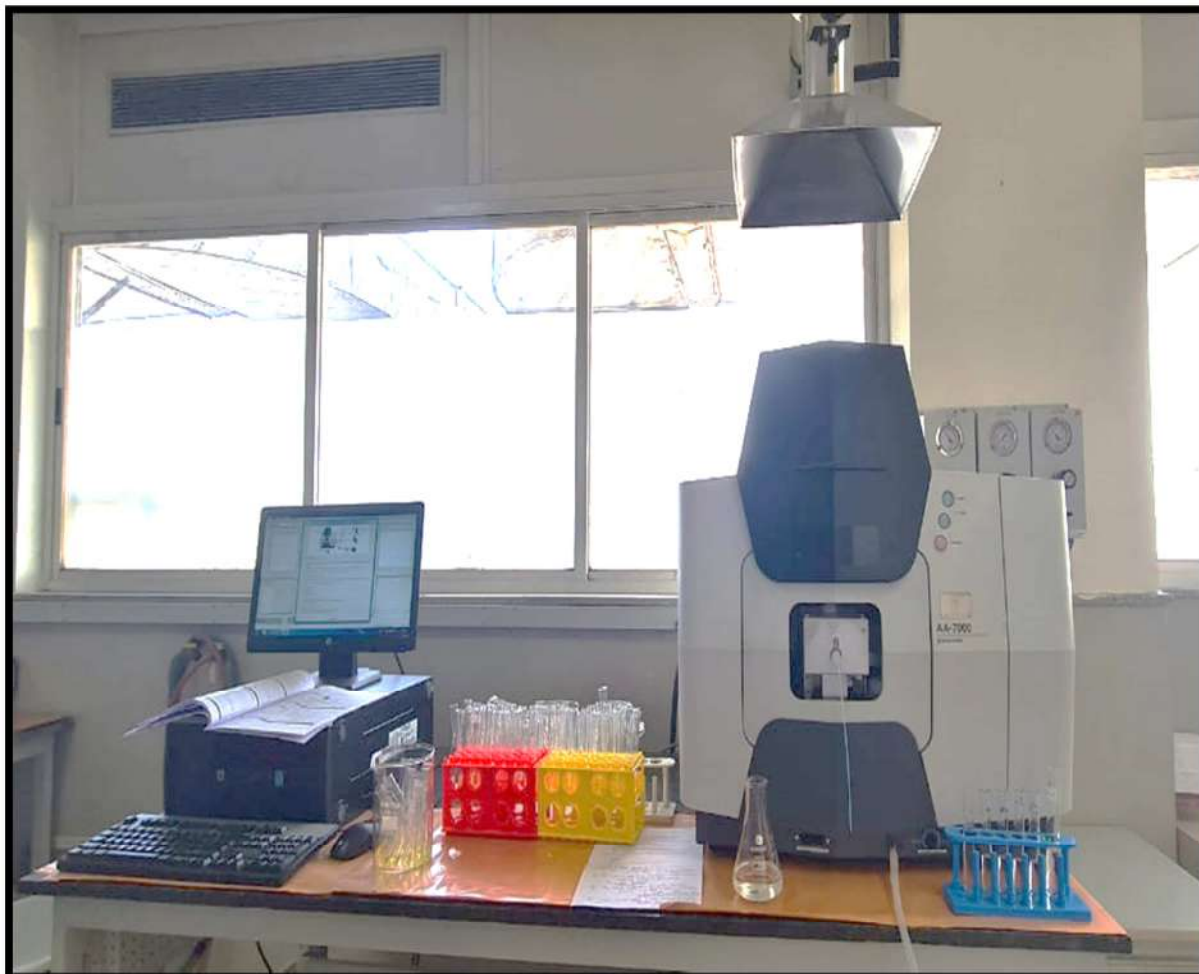
Photograph 5: THE SET UP OF FAAS – AA-7000 SPECTROPHOTOMETER WITH THE ASC-AUTOSAMPLER AND THE WIZAARD SOFTWARE BEING USED TO TEST ALL THE SAMPLES
