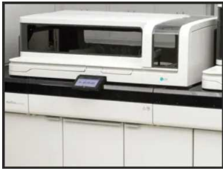
ATELLICA analyser for measurement of urinary beta 2 microglobulin
