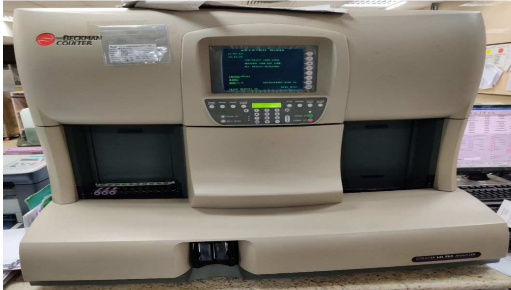
Beckmann coulter used for analysis of complete blood picture
