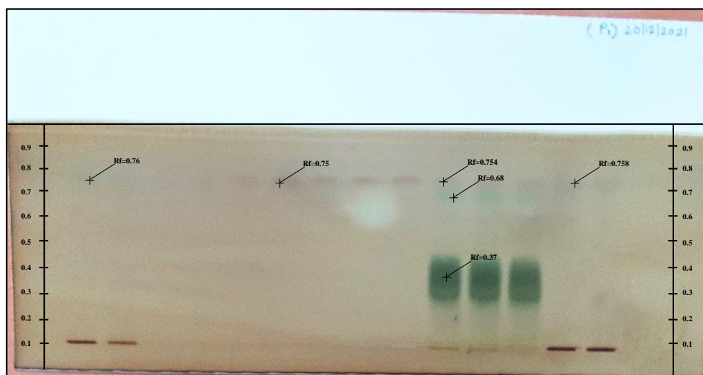
Fig.74: Gallic acid, T. arjuna and Ayurvedic formulation derivatized with Vanillin reagent (Plate Image @540 nm)
