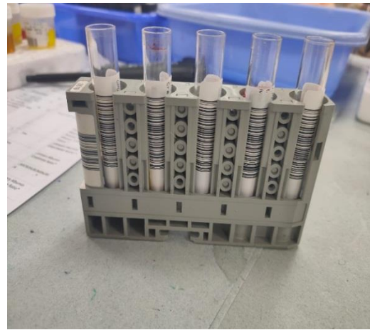
After serum separation the samples are arranged in sample rack for placing the rack in the analyser for estimation
