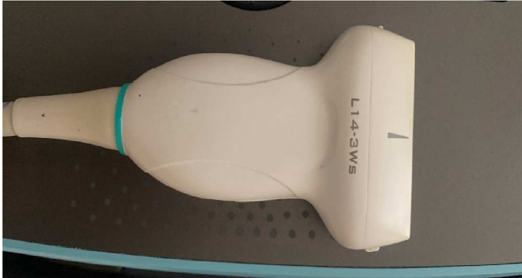
L14-3WS High frequency linear array transducer
