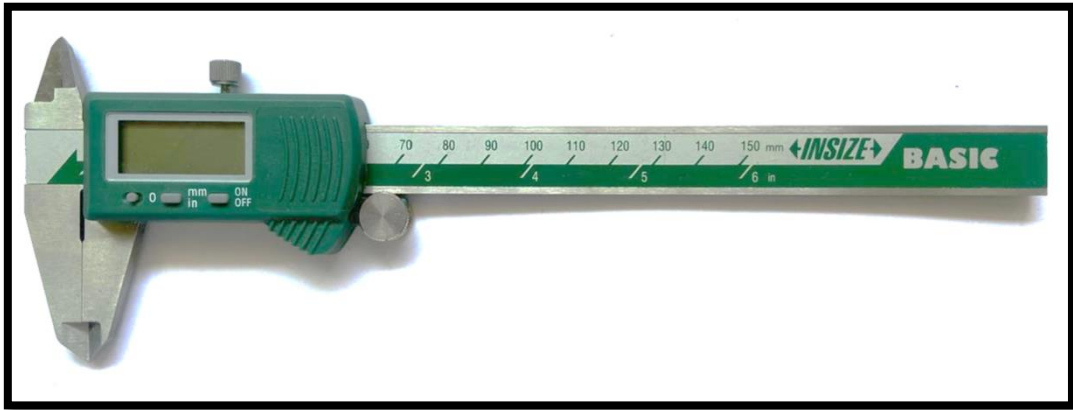
Picture 3: INSIZE digital vernier caliper used in the study.
