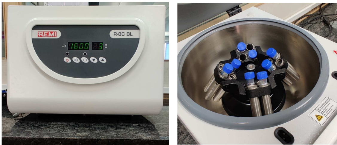
Picture 4a and 4b: Centrifuged at 400–500 × g for 25–30 minutes at room temperature without brake
