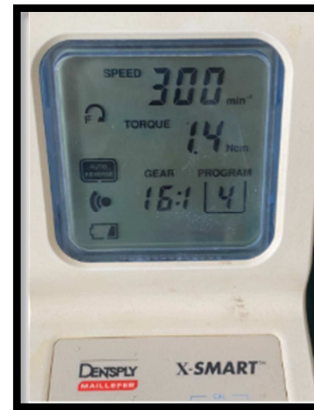
Fig.19 Speed and torque Neolix Neoniti rotary file system
