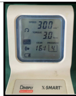
Fig.21 Speed and torque E3 Azure rotary file systems
