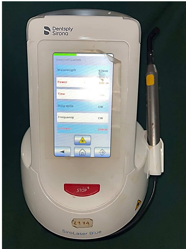
Fig 28 Laser parameters at 970 nm settings
