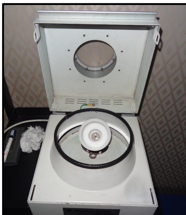
Fig 5. The dual axis container holder of Hauschild SpeedMixer DAC 150.1 FVZ
