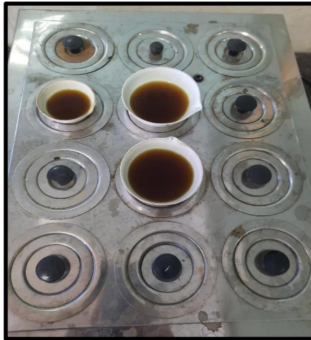
Figure 7: Water bath used for evaporation of Anethum graveolens extract.
