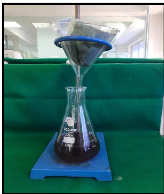
Figure 6: Crude extract filtration using Whatman No 1 filter paper
