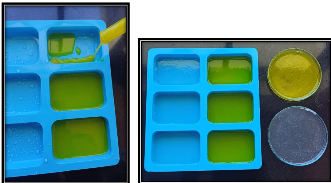
Figure 12: Polymer solution being poured for film formulation onto silicone molds and petri plates
