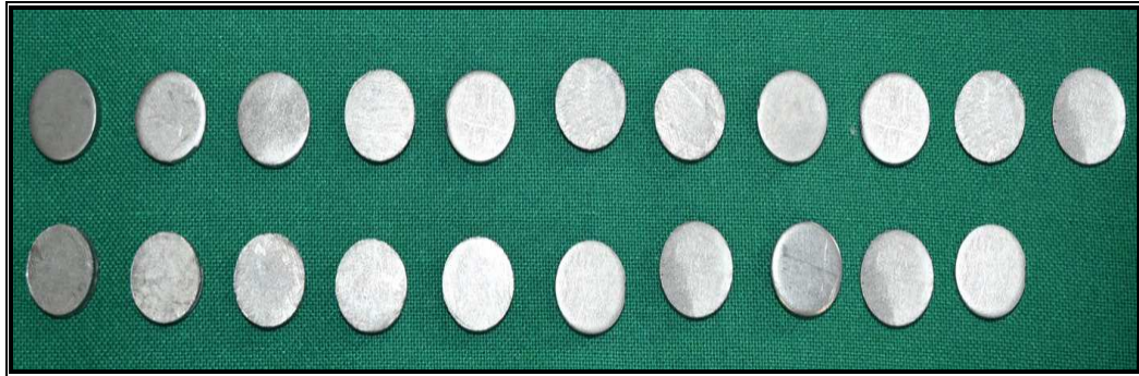
FIGURE 2: GROUP B – ALTERED TITANIUM SURFACE WITH NANOTUBES
