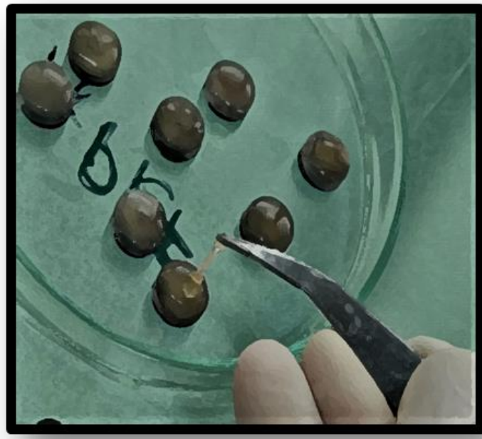
FIGURE NO 6: COATING OF TITANIUM DISCS WITH PLATELET RICH FIBRIN BY DIPPING METHOD
