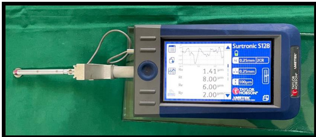
FIGURE NO 2: QUANTITATIVE EVALUATION OF SURFACE ROUGHNESS OF SPECIMEN USING PROFILOMETER
