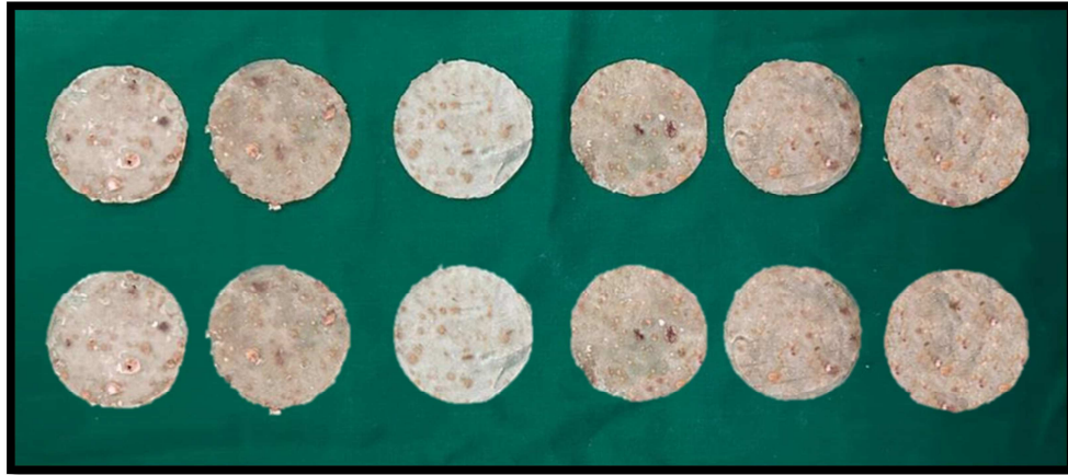
Figure 22: Specimens of 15% G. glabra group for water sorption and solubility for day 1
