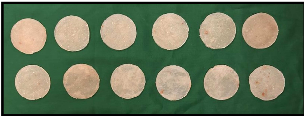
Figure 20: Specimens of 10% G. glabra group for water sorption and solubility for day 7
