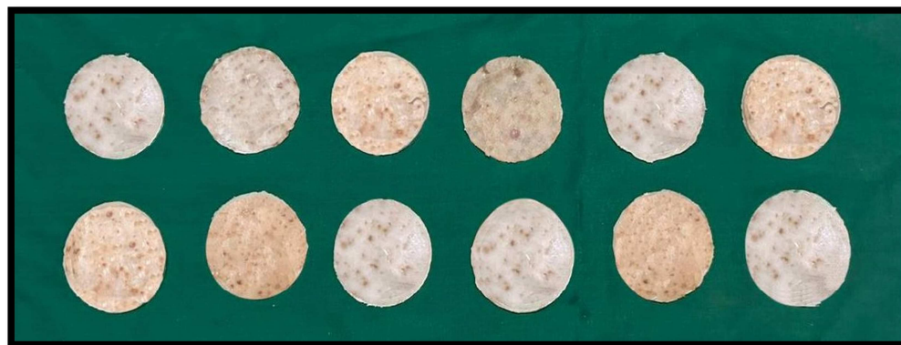
Figure 24: Specimens of 15% G. glabra group for water sorption and solubility for day 14
