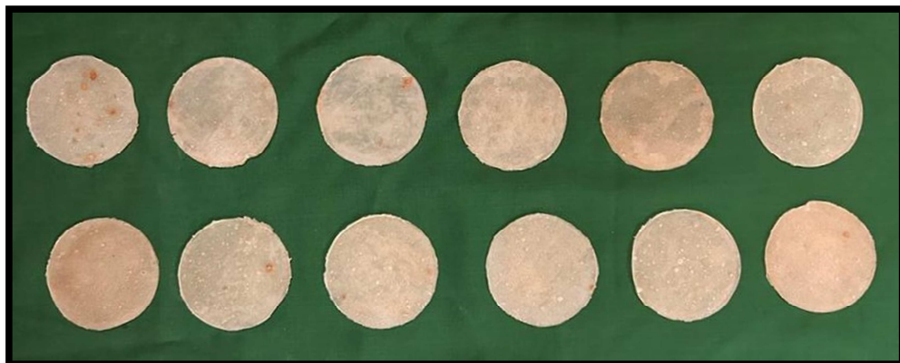
Figure 21: Specimens of 10% G. glabra group for water sorption and solubility for day 14
