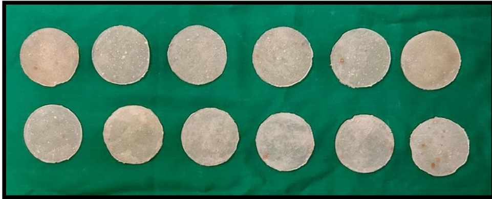
Figure 19: Specimens of 10% G. glabra group for water sorption and solubility for day 1
