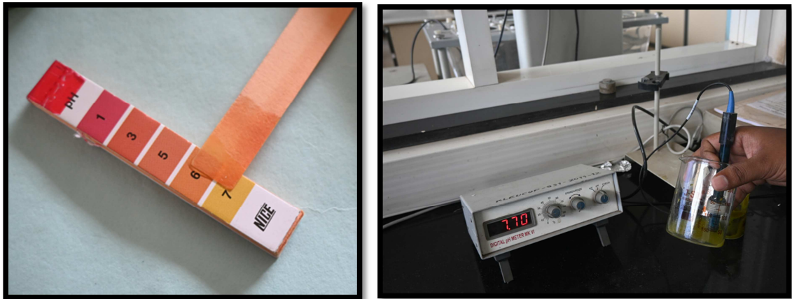
Fig 16: Adjusted pH is verified by digital meter
