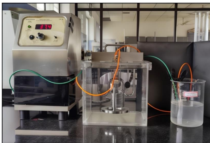
Figure 4: USP (Type IV) flow through cell dissolution apparatus.
